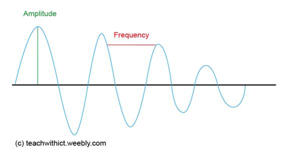
The amplitude controls how loud the sound is and the frequency controls the pitch.
